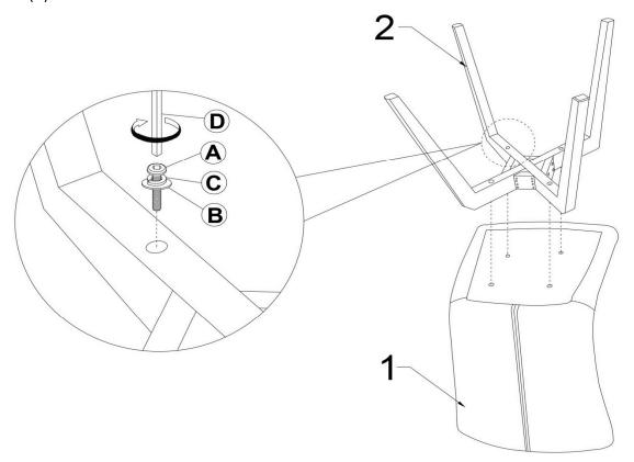
**IMPORTANT NOTE** - BEFORE FINALLY TIGHTENING THE BOLTS, PLACE THE ASSEMBLED CHAIR UPRIGHT ON A LEVEL SURFACE AND SIT CAREFULLY ON THE CHAIR TO ENSURE THE CHAIR LEGS ARE ALIGNED AND LEVEL. THEN TIGHTEN ALL BOLTS AND YOUR CHAIRS IS READY FOR USE.
